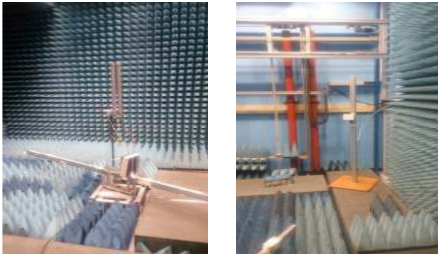
Fig. 4: Array measurement in GBSAR anechoic chamber experimental setup inside the chamber saved. The phase shifters were controlled using ESP8266 thing module programmed in arduino IDE. Four measurements were performed for the required phase states of Table I.
