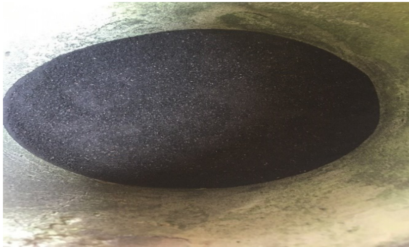
Figure 1: Partially burnt Rice Husk ash
