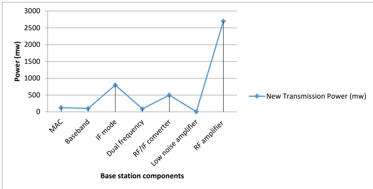
**Fig. 8:** Analysis of the energy consumed by the base station components with hibernation model during transmission process
