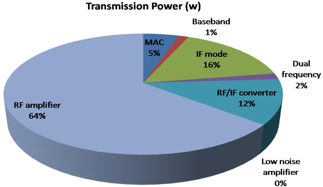
Fig. 9: Percentage energy consumption of the system by individual components
