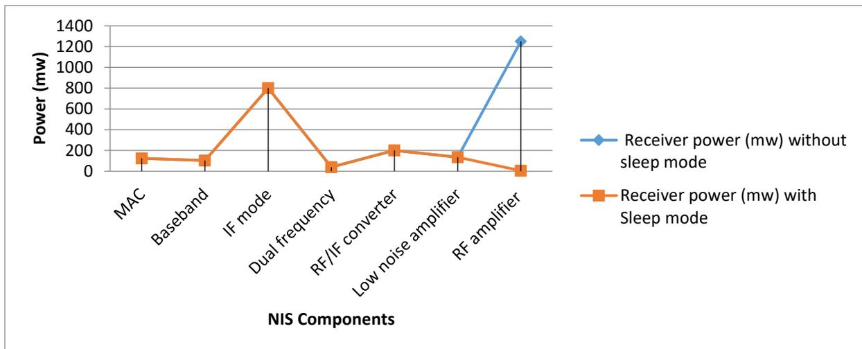
**Figure 13: Comparative receiver power**
