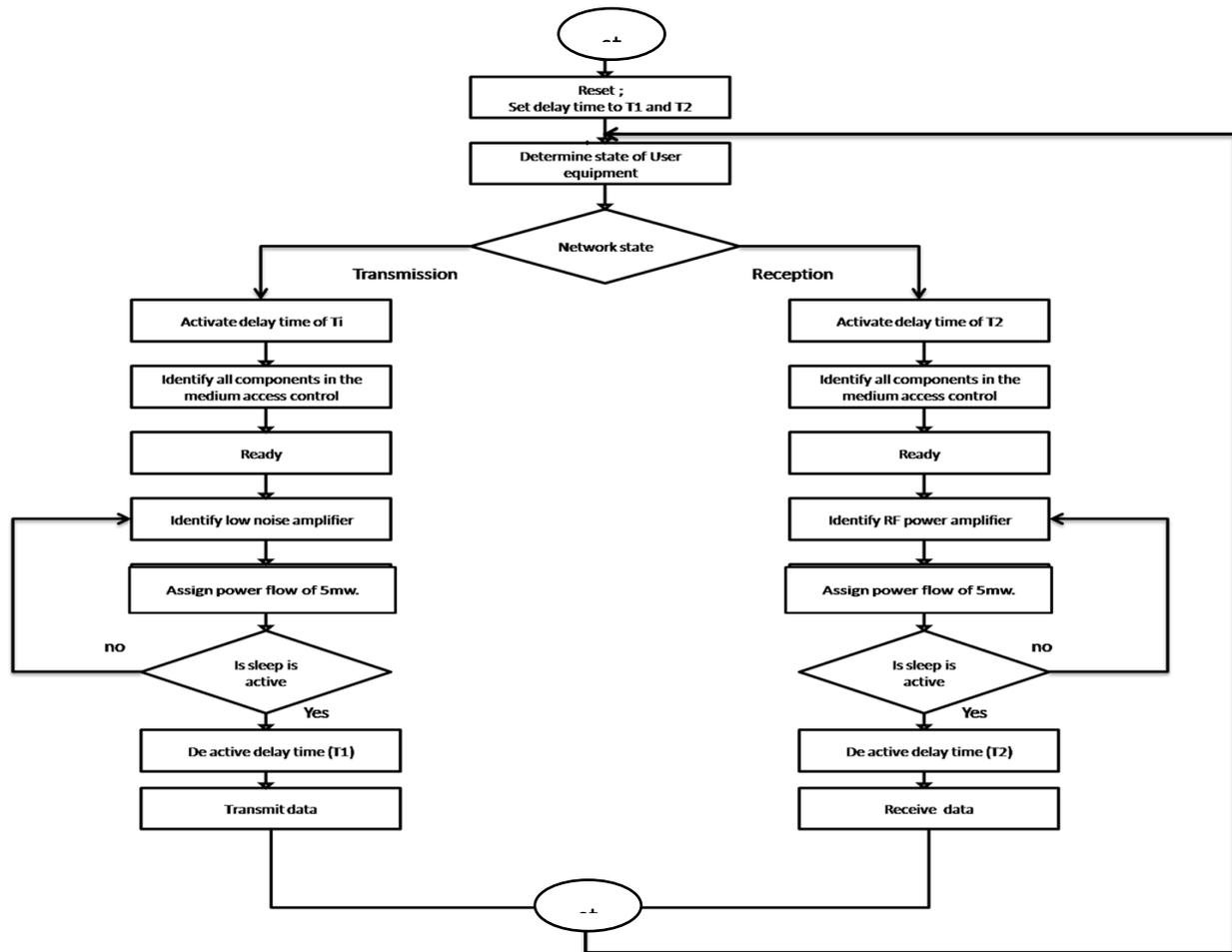
Fig.6: Model for inactive component hibernation process
