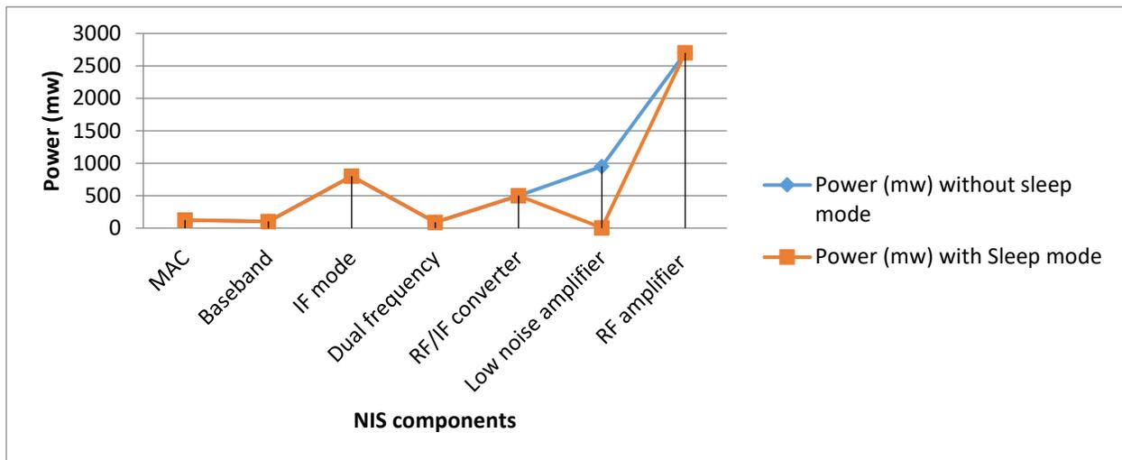
Fig. 12: Analysis of the energy saving effect of hibernation scheme on the communication base station during the transmission process
