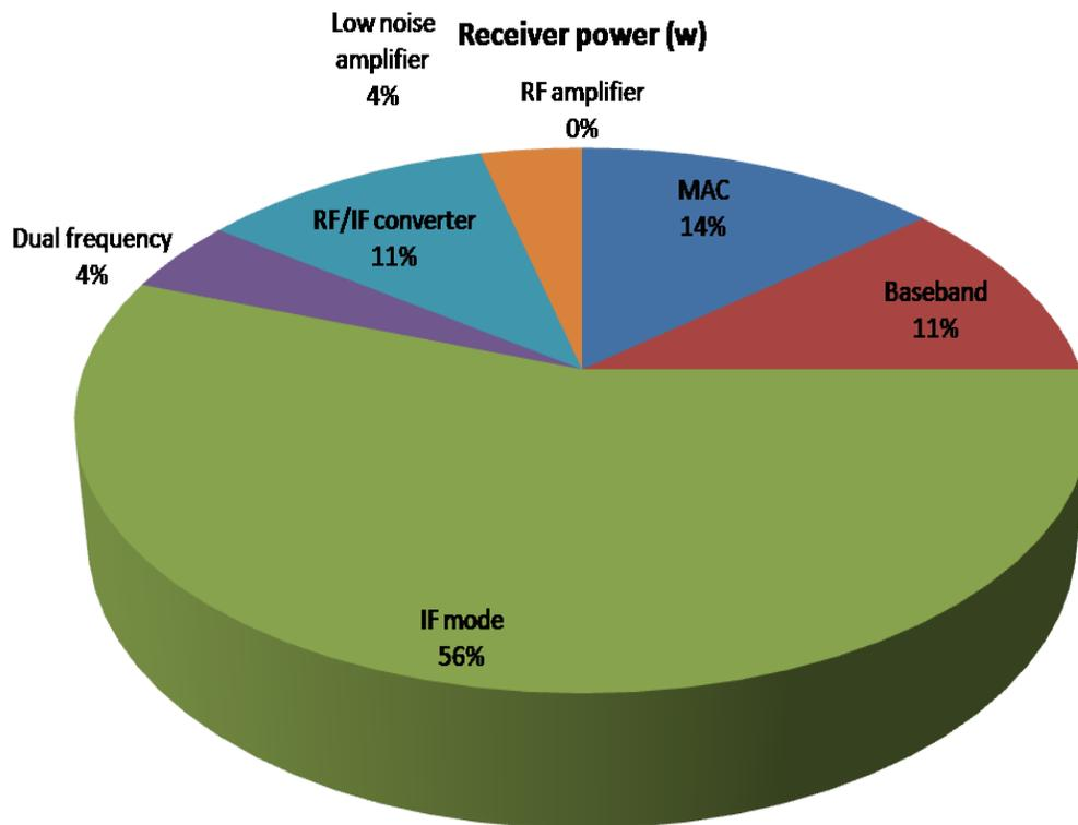
Fig. 11: The performance analysis of the overall power consumed at receiver end
