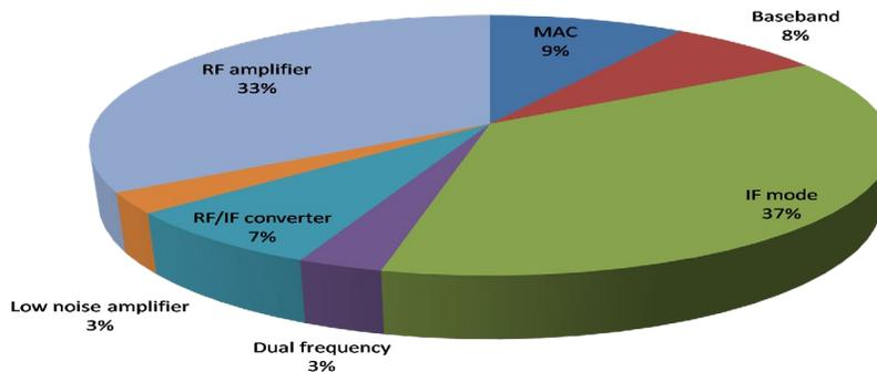
Figure 5: Power consumption rates of the base station components by the receiving nodes
