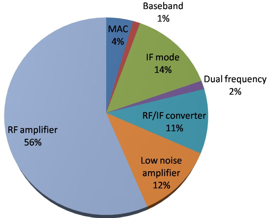
Figure 4: power consumption rates of the base station components by the transmit nodes
