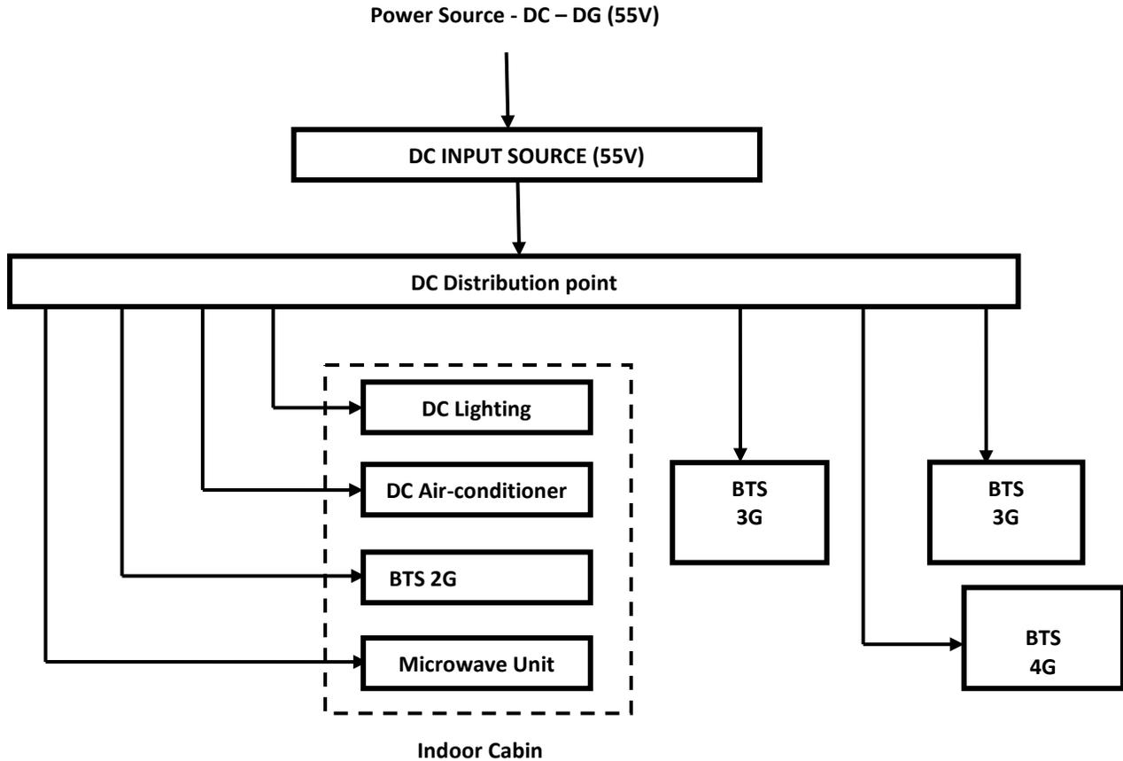
**Fig. 2:** Block Diagram of Power supply Architecture of the base station
