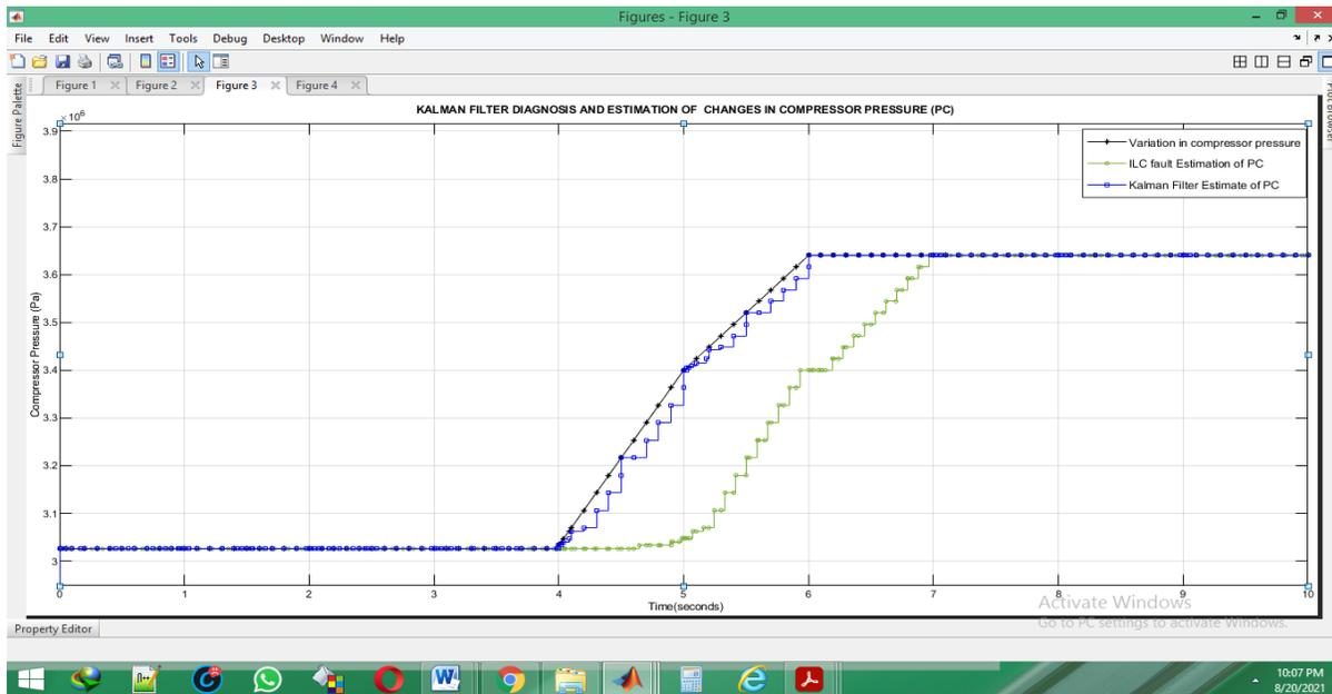
Figure 12: Changes in compressor pressure during component fault condition
