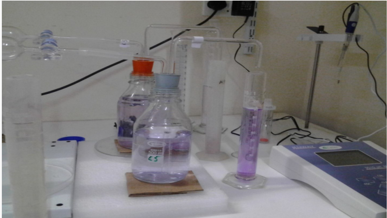
Fig. 1: Measurement of Methane Volume by Downward Displacement of Water Technique
