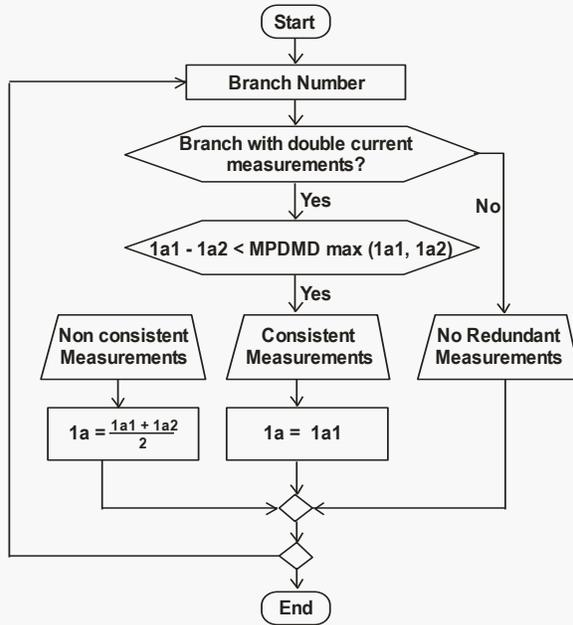
**Fig. 1: Flowchart of the algorithm for branch currents consistency check**
