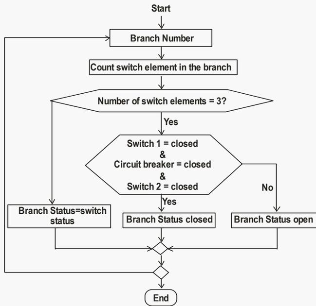
**Fig. 3: Flowchart of the algorithm for branch status determination**
