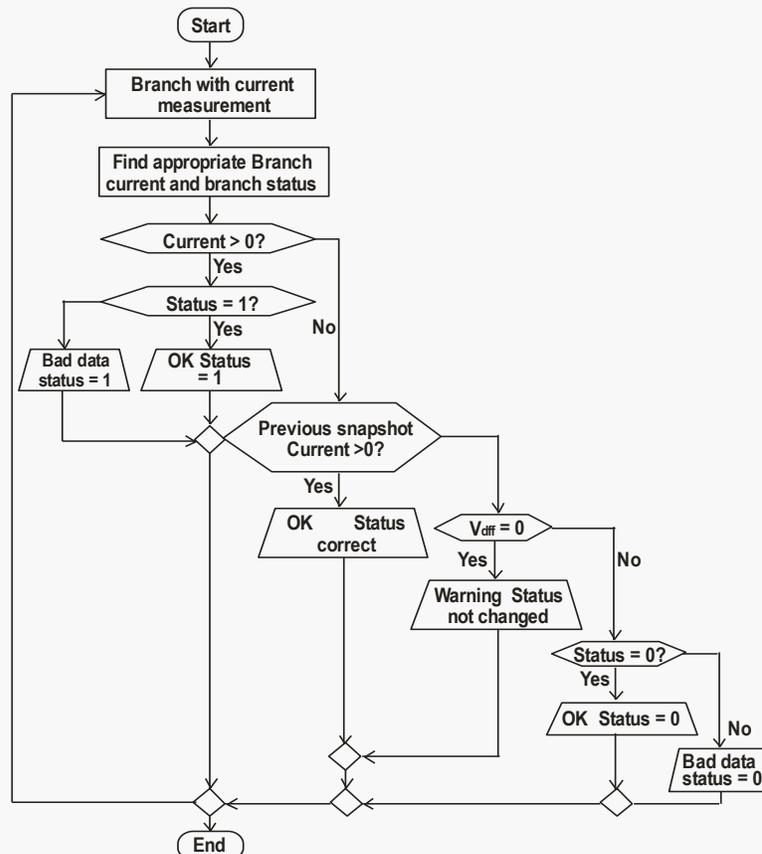
**Fig. 4: Flowchart of the algorithm for consistency check of branch current and status**
