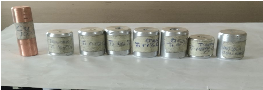
Figure 4: Developed beta phase Titanium copper specimens and copper specimen
