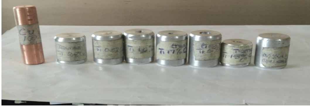
Figure 3: Developed beta phase Titanium copper specimens and copper specimen
