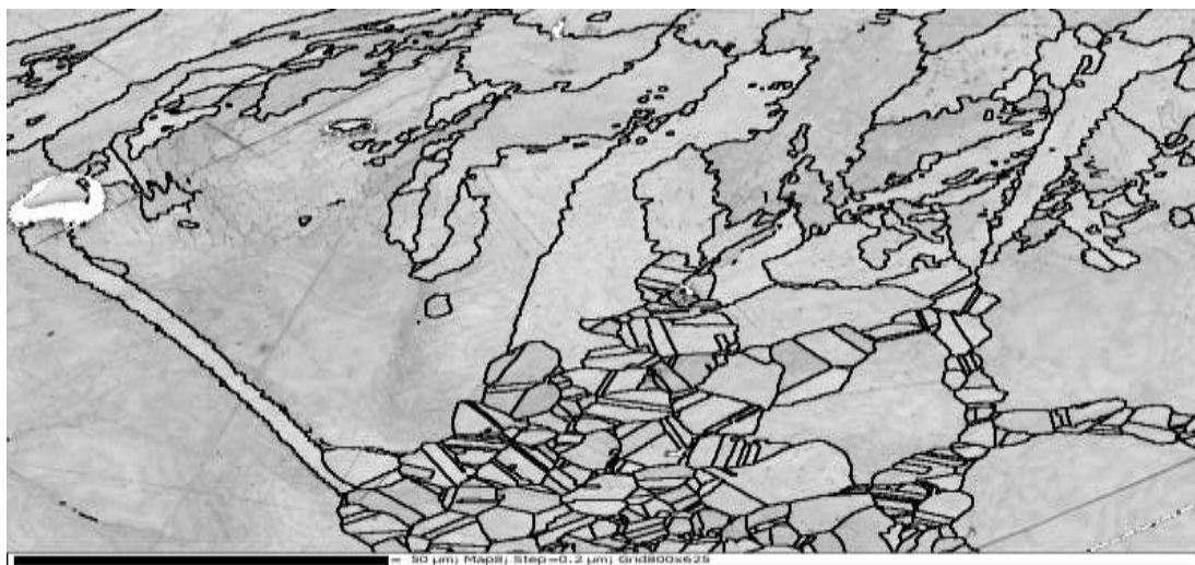
Figure 7: Band contrast map of EBSD for substrate and laser regions
